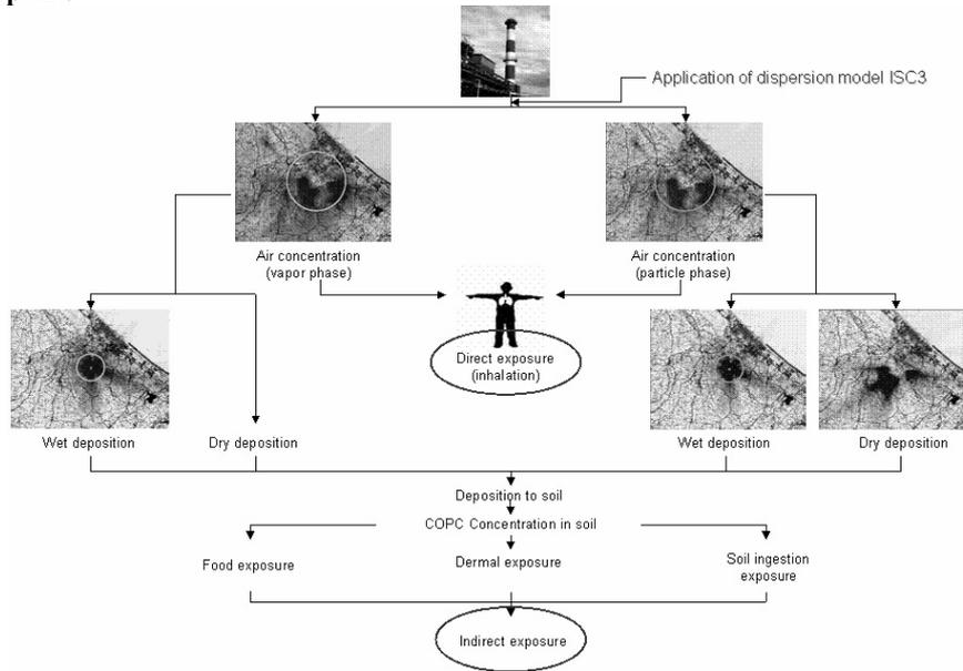
**Fig. 8 - Atmospheric dispersion of fine particulate (PM<sub>10</sub>) from an incineration plant.**
